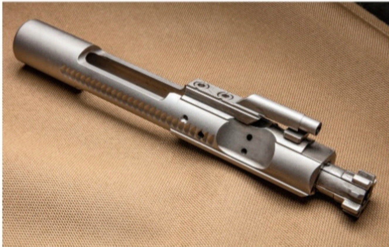
The bolt carrier group features a 4340 heat-treated cam pin, and an 8640 heat-treated firing pin. The extractor is precision ground 4340 and the ejector is made of S7 tool steel; both are heat treated, also.
