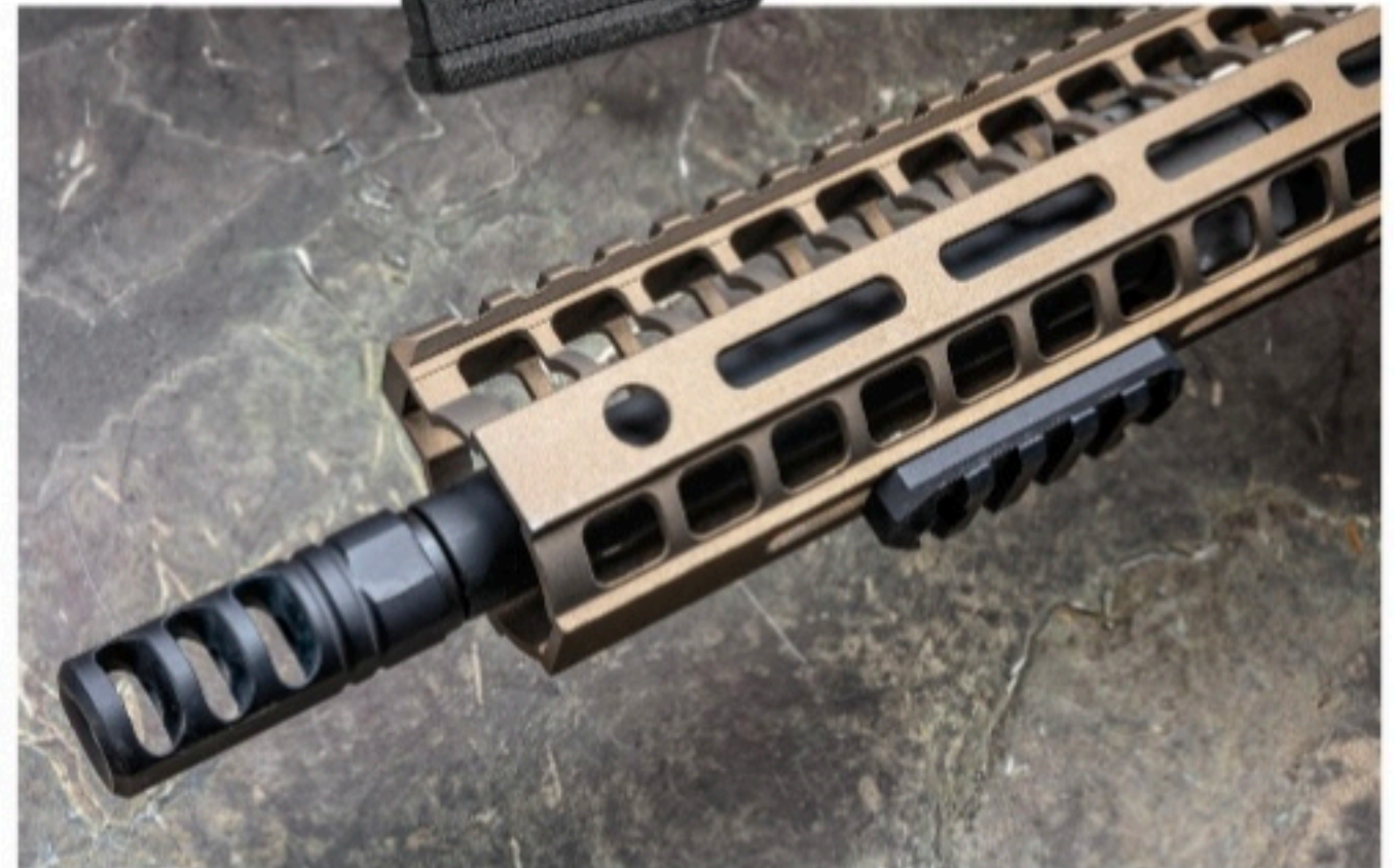
The ADER's mid-length gas system and barrel are shrouded by ATAC's proprietary handguard that features M-Lok slots to attach rail sections and accessories. The barrel is complete with a muzzlebrake.
