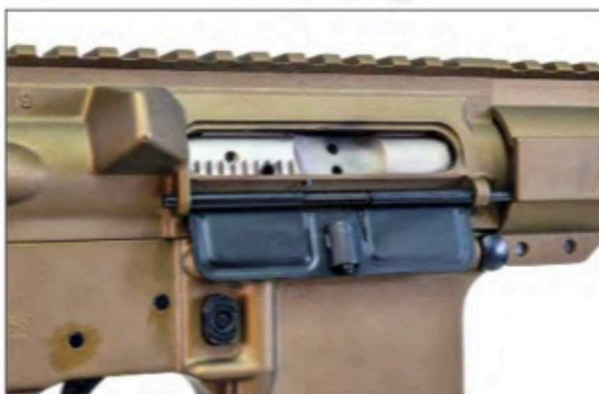
The nickel boron coating on the bolt/carrier keeps it slick, which helps to keep it running longer when it's dirty. It is far easier to clean than a standard bolt carrier.
