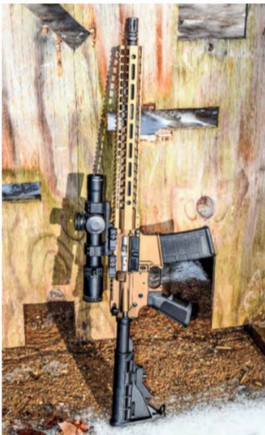
While Cerakoted rifles look cool, the main functional advantage to a non-black rifle is that they don't get too hot to touch in the sun.
