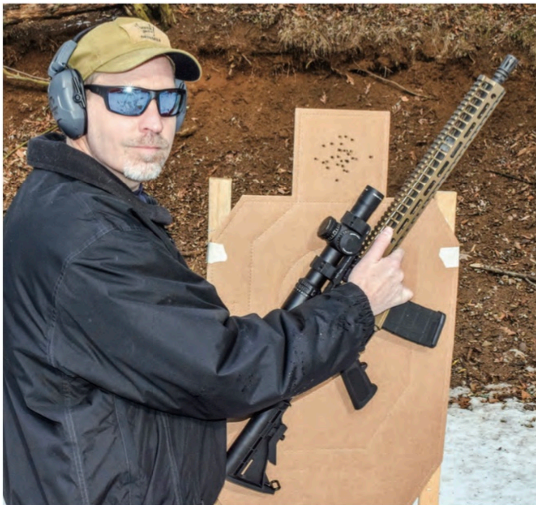
Low power variable optics (LPVOs) have their advantages. Firing from the standing, supported position (left forearm pressed against a vertical post), with the Trijicon AccuPower 1-8X cranked all the way up, Tarr put an entire 30-round magazine into the head of an IDPA target at 75 yards.
